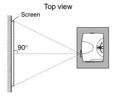
Point the lens straight at the center of the screen as above.
